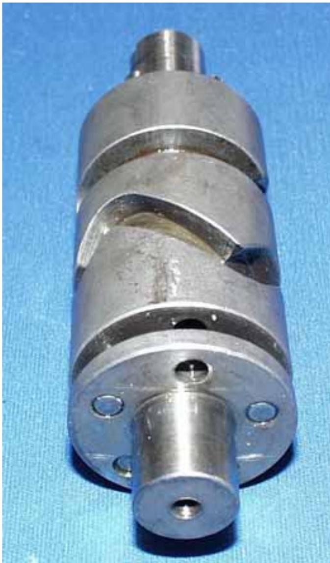
**Figure 3:** Lilac LS-18 shift drum with pin removed
