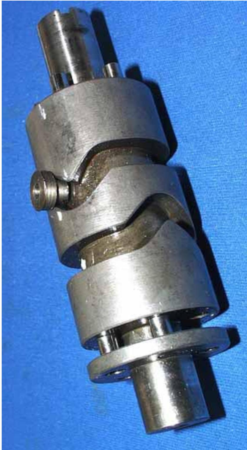
**Figure 4:** Drill bush in position
